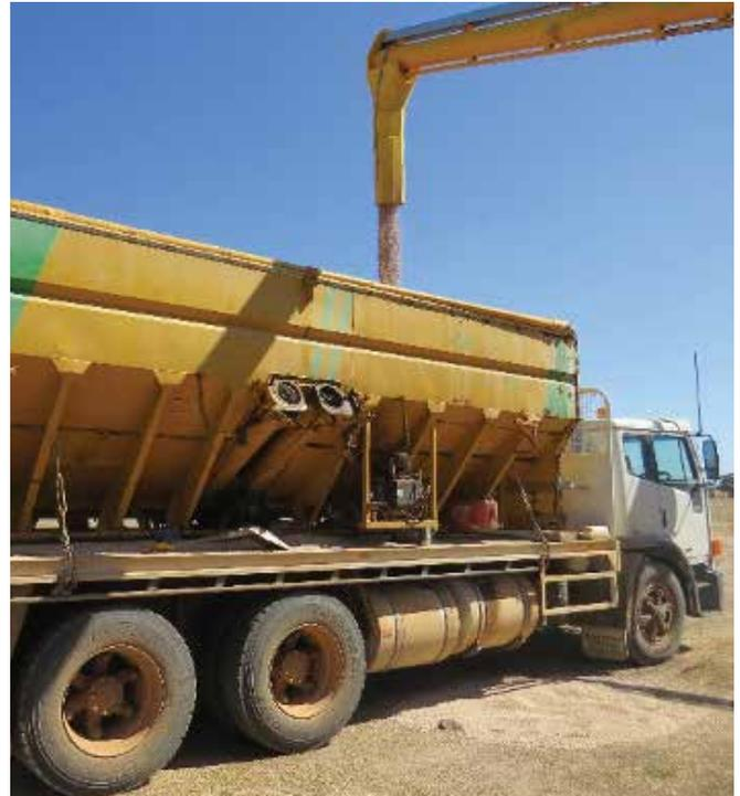
Shows the feed truck with Cole bin mounted on load cells being filled with lupins.
