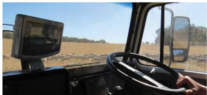
Monitor display in the cab shows grain weight which allows for accuracy of feeding.
